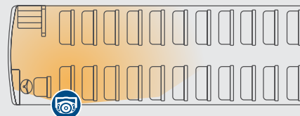
HD3U HD Ultra-wide Interior Camera 1.72mm Driver/ Step Well View
