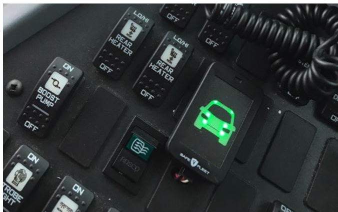
Display Module onboard bus indicating it is safe to cross
