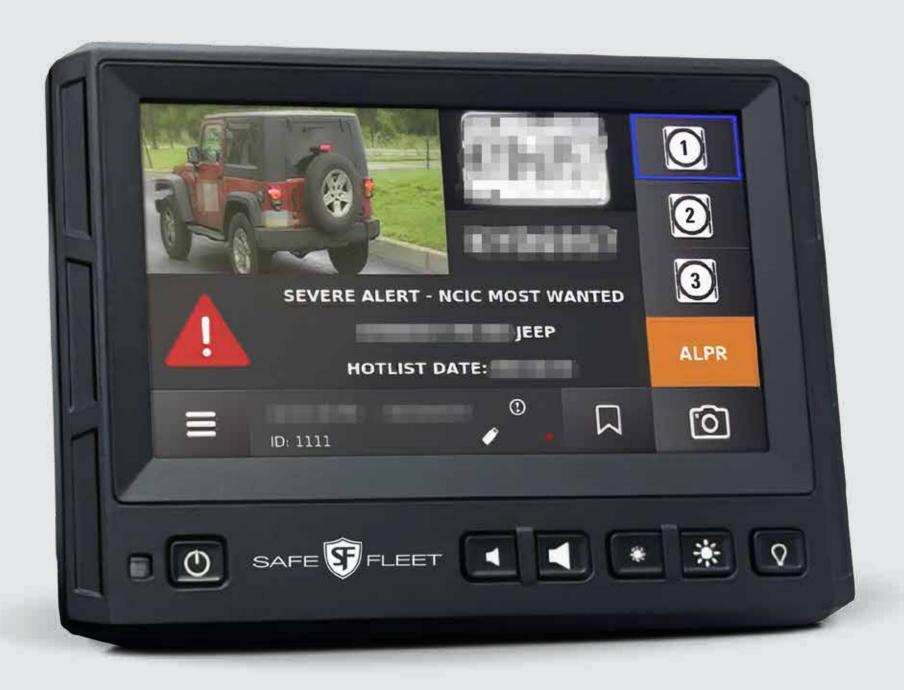
Safe Fleet FOCUS H2 with ALPR is a new Automatic License Plate **Recognition system** (ALPR) that does not require separate hardware—it works in the background of the FOCUS In-Car Video System and notifies officers of hotlist matches as they occur.
