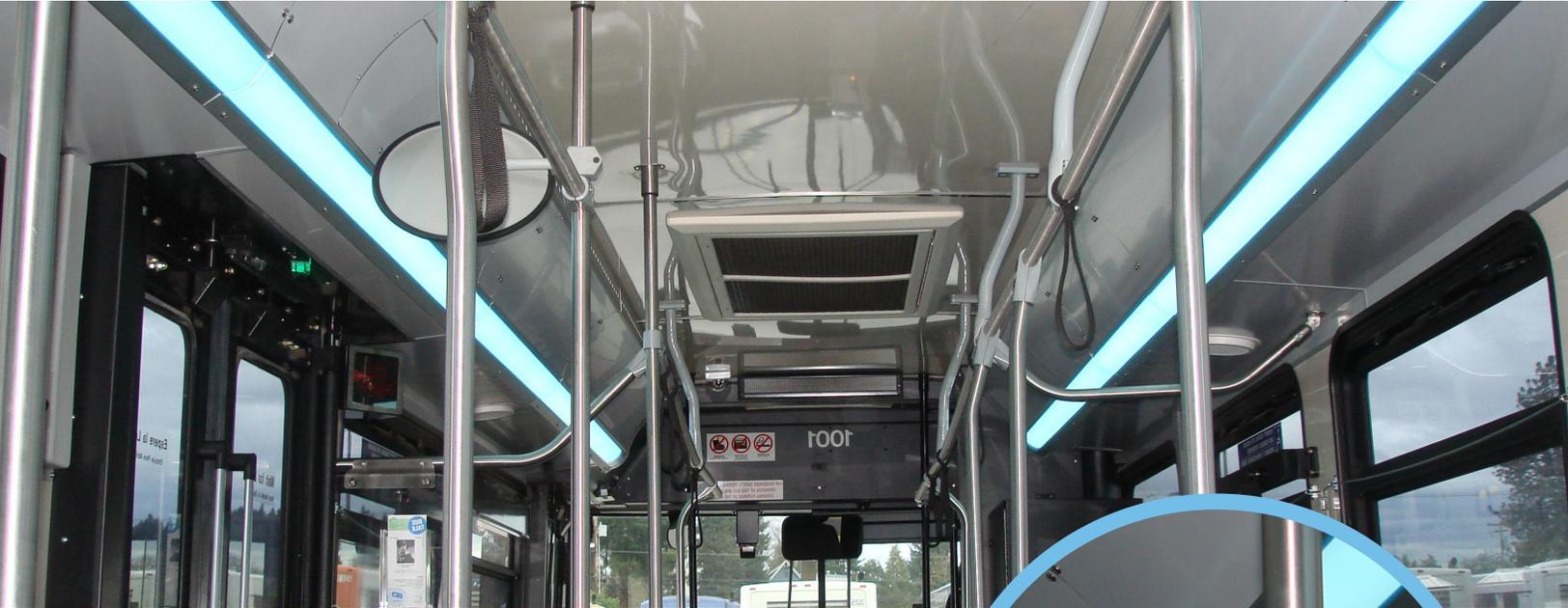
Interior LED lighting with dimming options per system. Lighting output configurable based on desired preferences.
