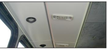
Ducted OPR (Dual Reading Lights / Adjustable Air Vents)
