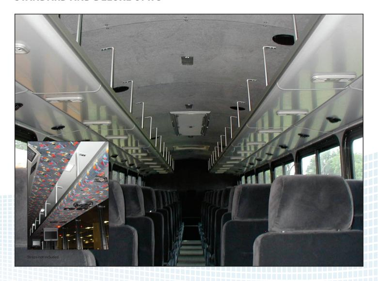
Designed and manufactured for each individual bus model providing unique and cost effective solutions. Pretoria pioneered the use of lightweight aluminum composite panels in conjunction with satin anodized aluminum extrusions to provide solid and easy to install systems. All of our OPR's systems are available with integral ducting that is engineered for use with all types of AC units.
