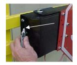
1. Using a utility knife, cut the silicone seal on both ends of the stop arm cover. using 5/16" socket
