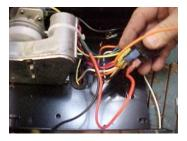
7. Reattach the red and black motor wires to the relavs (or to module- if 6-series). The red wire attaches to the upper relay, the black to the lower.
