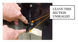
8. Replace cover. Secure with (2) screws. Reseal both ends of the crossing arm cover with RTV. IMPORTANT! - DO NOT seal approximately 1" of the lower right side of the box. This provides an additional drainage location. Test the assembly to make sure it functions correctly.
