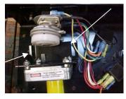
5. Remove (2) each of washers, lock-washers and nuts on the motor bracket and remove both the motor and bracket from the assembly, using a 7/16" socket
