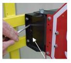
3. Remove the cover by using a flat bladed screwdriver to pry it off.
