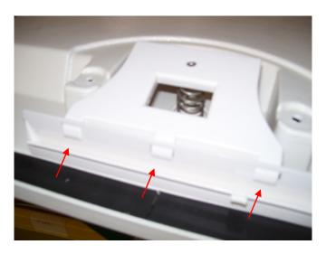
**STEP 9.** Place the new handle/spring on the lid. Ensure that the handle hooks are in the openings of the handle base (3 places).
