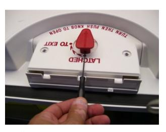
**STEP 2.** Orient the inner red knob as shown. Remove set screw in knob using 5/32" allen wrench.
