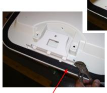
**STEP 6**. Remove the hinge pin from the side of the handle base. Pushing on the handle makes it easier to remove the pin. Caution: gloves are recommended for this step as plastic edges can be sharp.
