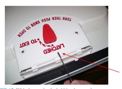
**STEP 15**. With the two knobs held in place as shown, secure the set screw in the inner knob. After tightening the set screw, rotate the knobs 180° until the inner knob's arrow points to "LATCHED".
