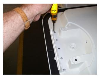
**STEP 7.** Using a T-20 Torx bit, remove the 5 screws that hold the handle base to the lid.
