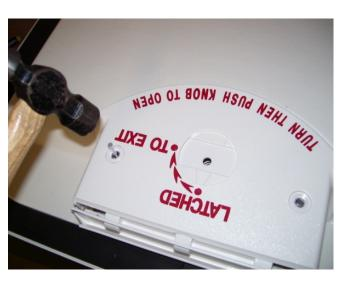
**STEP 12.** Hold the handle shield down against the lid. Insert the rivets into the holes in the shield and the holes in the lid. Lightly tap on the head of the rivets to set the rivets.
