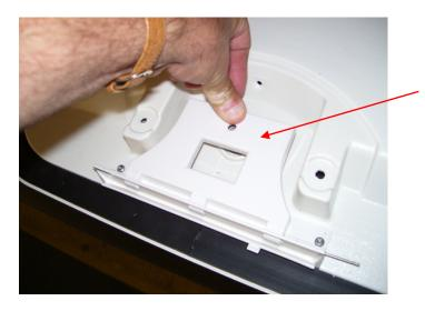
**STEP 10.** While pushing down on the handle, slide the hinge pin into the hole on the handle base. Pushing on the handle will help locate the pin during insertion. You will need to guide the pin into the second hole on the handle from underneath the handle. Lightly tap the pin with a hammer until the pin is fully inserted.
