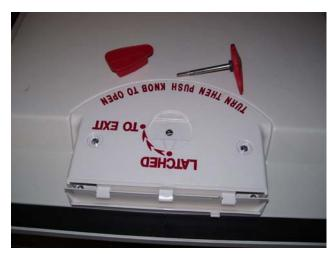
**STEP 3.** Unscrew the inner red knob from the outer red knob. Remove each from the lid.
