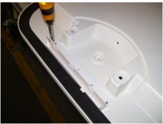
**STEP 8**. Using the same screws, attach the new handle base to the lid.
