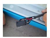
Place new switch and wire harness into switch cover
