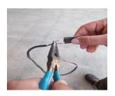
With a pair of needle nose pliers gently walk the wire and terminal off of spade connector
