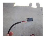
The pigtail is attached to the switch by spade connectors (1) Remove the existing wires from switch
