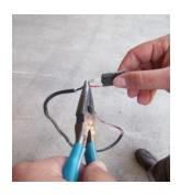
Using needle nose pliers remove top connector
