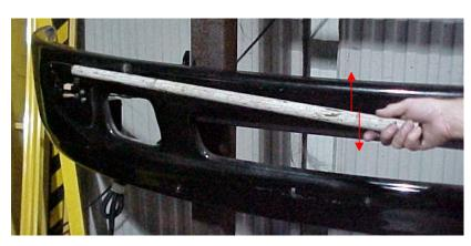
4.) Slide a pipe over the arm protruding through the slot in the bumper and push up or done slightly as required. Fit yellow poly rod over to see if aligned & contacting magnet. If arm is in position install ¼-28 bolts and formed washers. If arm is still out of–line, remove yellow poly rod and bend again slightly using the pipe. Install yellow poly rod.
