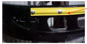
1.) THE CROSSING ARM WILL BE IN THE FULLY CLOSED POSITION AS SHOWN IN PHOTO TO LEFT, BUT THE UNIT WILL CONTINUE TO RUN.
