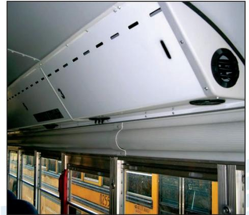
Our design team works closely with the bus OEM, the AC OEM and the customer to provide air moving systems that are both functional and aesthetically pleasing. For example, our vacuum forming and mold construction processes ensure the ABS end caps provide an excellent "fit and finish".
