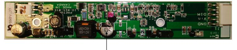
The presence of one capacitor will result in a 20% light output while in Dim mode.
