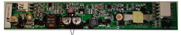
The presence of two capacitors will result in a 10% light output while in Dim mode.
